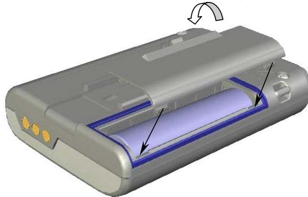
To replace the battery door, firstly locate the door lugs into the positions shown and then rotate the door downwards, closing the door loosely. Further compress the door at both ends simultaneously and push down until the door clicks shut, compressing the battery and surrounding gasket.
