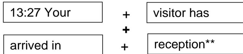
If a call is cancelled during the alert period, the MUTE button may be used to review the message and to speed-up, or slow-down, the viewing process. If MUTE is pressed and held, the message is held at the current screen; releasing MUTE causes the next screen to be displayed. If MUTE is pressed and released during the final message screen, then the display will revert to the first part of the message and the whole message viewing process may be repeated.
