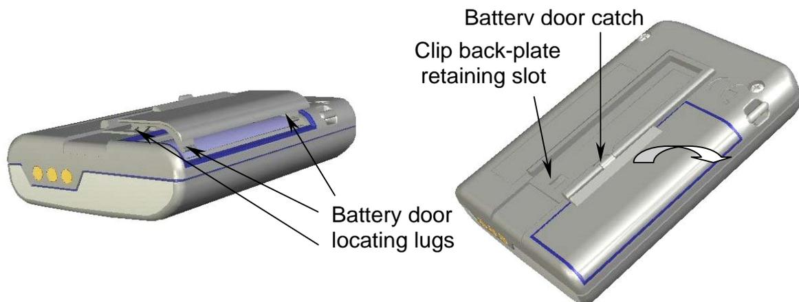
Ensure that the battery door lugs are lifted clear of the case and remove the door. Remove the battery by placing your forefinger onto the positive end-cap and lifting the battery upwards, at the same time pushing slightly backwards against the negative contact spring.
